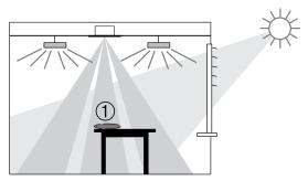
Room correction factor = Brightness value on the ceiling Brightness value on the work surface
