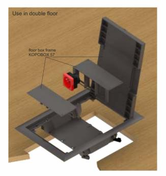
KOPOBOX 57 is designed for mounting of modular apparatuses 45 x 45. Installation of the classic apparatuses into this frame is not possible. However it enables the installation into floors already from a depth of 56 mm. The cover plate for apparatus for modular apparatuses is already a part of the frame KOPOBOX 57 and it is not necessary to order it separately.
