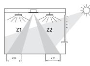
Each light measurement zone maps a rectangle of about 2 x 4 m on the floor. Depending on the selected the detection zone, the light measurements are assigned as follows:
