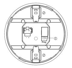
① Programming mode button② Mechanical safety lock
