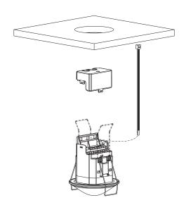
Installation in false ceilings for ceiling thicknesses of 0.5 mm to 3 cm. The diameter of ceiling cutouts must be between 62 mm and 70 mm. The cable strain relief is with using a cable tie (width: 3.5 - 4.8 mm).
