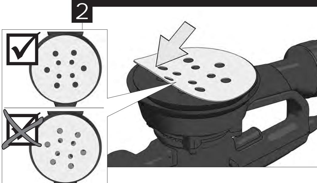
Press carefully the fuzzy side of sanding disc against the packaging pad, as firmly as possible.
