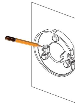
Use a 6 mm drill bit to make the required holes approximately 25 mm deep, then insert the wall anchors into the holes. Use the screws provided to attach the mounting bracket to the wall.
