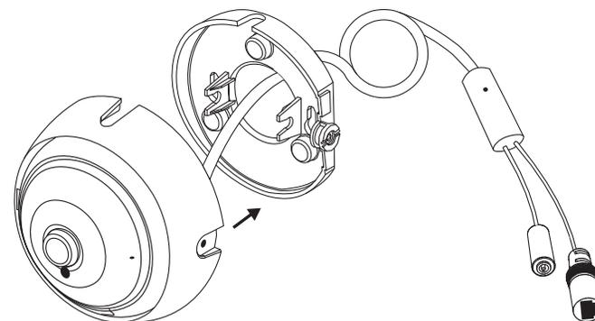
Adjust the angle of the camera, then screw in the tilt adjustment screw until it is snug.
