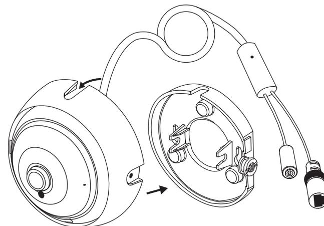
**If you wish to run the camera cables through the wall or ceiling,** pull the cables through the hole.
