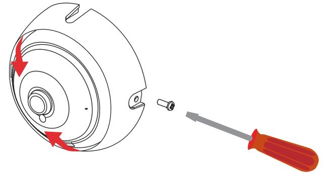
**If you wish to insert a microSD card**, remove the camera from the camera mount by turning the camera counter-clockwise and lifting it away from the camera mount.
