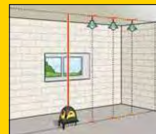
Plumb line – take a point from floor to ceiling
