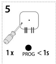
Press of programming button on receiver RFSAI-61B shorter than 1 second will finish programming mode (LED switches off).
