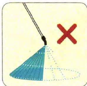
Clean nozzles and filters
