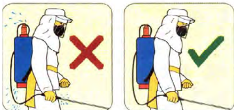
Check for damage and leaks
