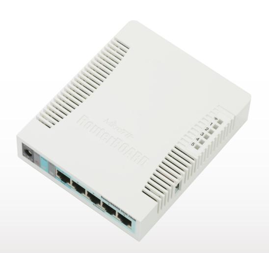
The RB951G-2HnD is a wireless SOHO Gigabit AP with a new generation Atheros CPU and more processing power. It has five Gigabit Ethernet ports, one USB 2.0 port and a high power 2.4GHz 802.11b/g/n wireless AP with antennas built in.
