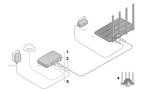
4. Connect the power adapter to the router and turn on the router.
